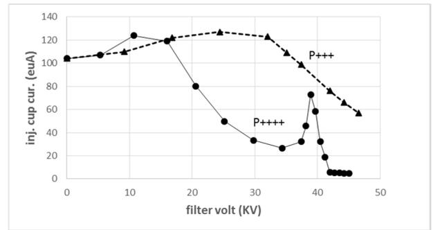
Fig. 6. Transmitted ions through retardation filter.
