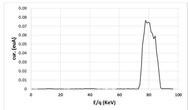
Fig. 4. Electrostatic rigidity spectrum of high current As++++ beam.
