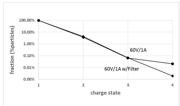
Fig. 8 Arsenic charge fractions. With and without the filter.
