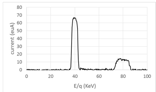
Fig. 3 Electrostatic rigidity spectrum of P++++ beam.
