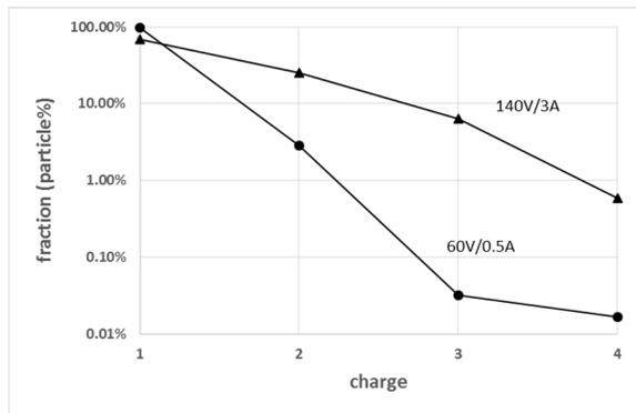
Fig. 2. Measured arsenic charge state distributions at two arc conditions.
