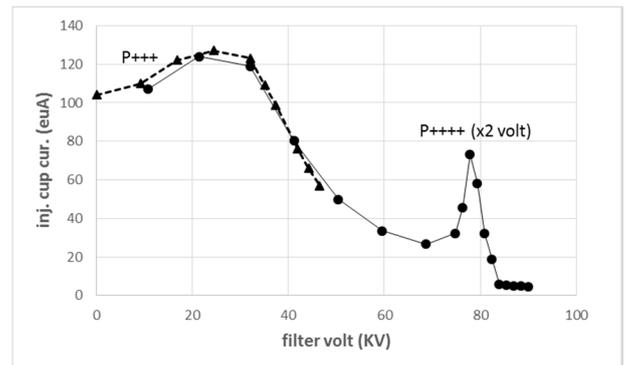
Fig. 7. Transmitted ions through retardation filter with doubled voltage scale on  $P++++$  data.
