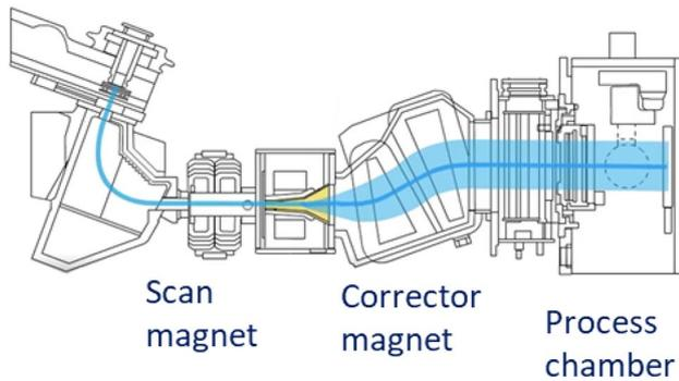
**Fig. 1** Overview of the Axcelis Purion® H hybrid scan high current beam line, where a mass resolved spot beam is scanned into a divergent beam via a scan magnet. After the scanning magnet, the divergent beam appears to originate from a vertex, and the beam is subsequently parallelized by a corrector magnet focusing the vertex to infinity
