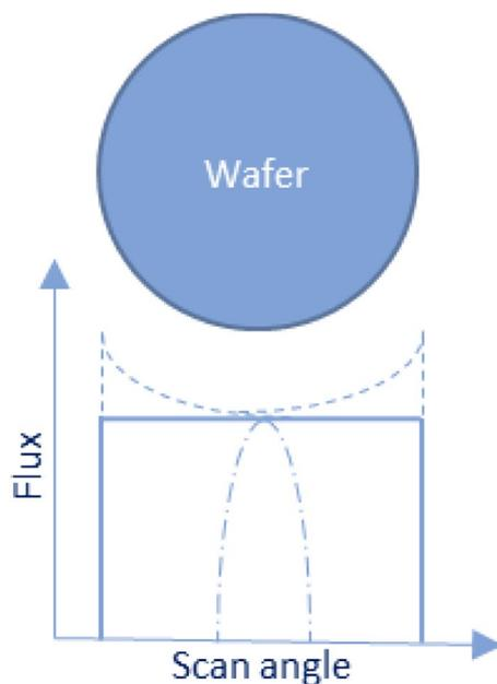
**Fig. 2** Flux distribution of the scanned beam for constant scan speed (dashed line) and with corrected scan waveform (solid) for a spot beam with finite width (dotted-dashed line)
