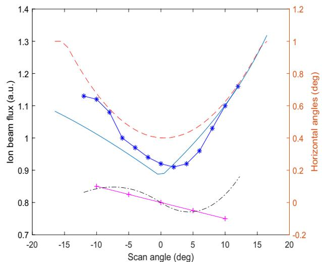
**Fig. 4** Comparison of desired (dashed line), model optimized (solid), and measured flux distribution (solid with stars) on a prototype corrector magnet, and horizontal parallelism (predicted=dot-dashed, measured=solid with crosses)
