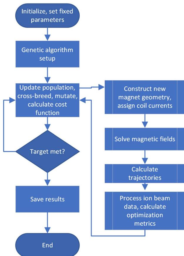
**Fig. 3** Flowchart for a genetic algorithm optimizing the design of a corrector magnet
