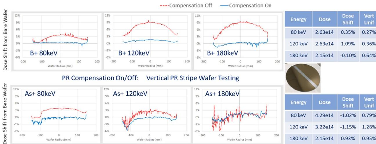
**Fig. 3** Vertical dose uniformity profiles obtained at different beam energies (80, 120, 180 keV) for 2-pass implants with Boron (Top half) and Arsenic (bottom half) at highest beam currents showing the excellent dose uniformity and minimal dose shift with implants
