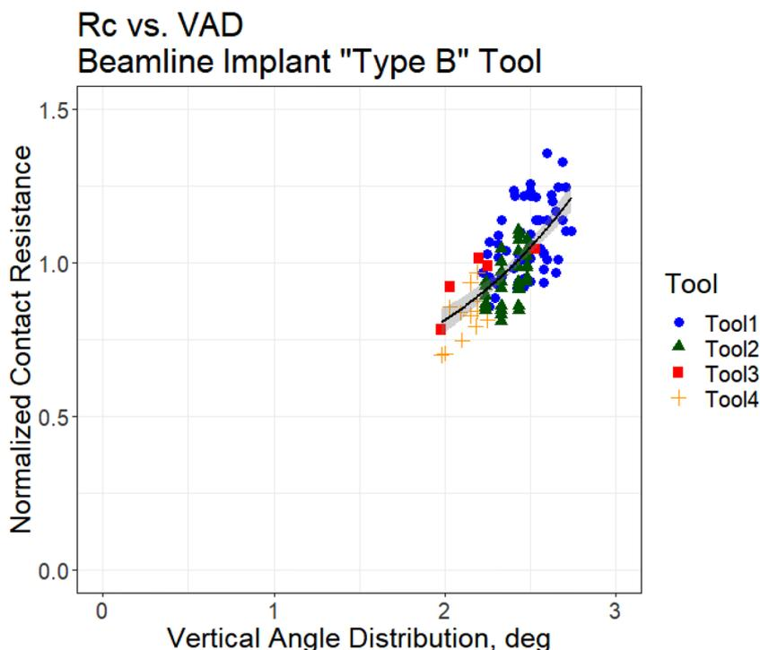
**Fig. 2** B<sup>+</sup> 3 keV ROI beam current is the scanned beam current in the wafer area. Tuning and hardware optimization are constrained to accept only solutions meeting several beam quality criteria: uniformity < 1%, VAD < 1°, HAD < VAD, ROI beam current between 12 and 14 mA with the Extraction Power Supply Voltage and Current held constant to within 0.2% and 2%, respectively
