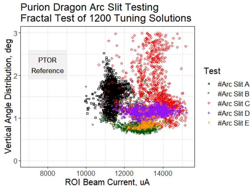
quad magnet tuning. When a new recipe is setup, a simplex routine is used to approach the minimum of this surface. Throughout the aging of the source the preferred method is to keep the quad magnet currents at their history values and tune only the gap between the arc slit and extraction electrode to find the minimum angle distribution as shown in Fig. 3b.
