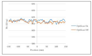
Fig.7. Vertical Rs line scans of glitch repainted wafers showing successful glitch repaintings with N=3 OptiScan.
