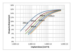
Fig. 6. An example throughput gain with OptiScan as a function of implant dose and beam current.
