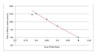
Fig. 5. Measured gain in scanned beam current density with OptiScan as a function of narrow scan width (R). Interlace ratio =2.
