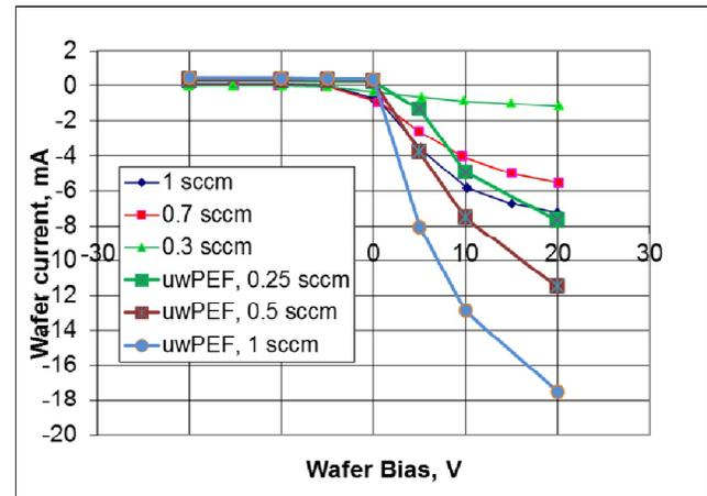
**FIGURE 4.** Net current to a biased wafer, no ion beam. For comparison, current drawn from a standard dc PEF (Xe-PEF, standard offering on Axcelis' Optima MD implanters, labeled std) is shown. Current delivered by our microwave PEF is labeled uwPEF.
