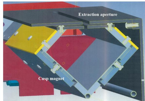
**FIGURE 1.** Cross-section of main PEF chamber housing the ECR discharge. Cusp magnet arrays line the lower walls of the chamber, and the whole assembly is water-cooled. PEF plasma is extracted through an extraction slit the width of the scanned beam.
