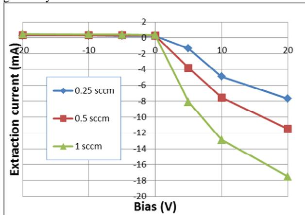
**FIGURE 3.** Current extracted from the PEF extraction slit by biasing the chamber. PEF power  $\sim 30$  W.
