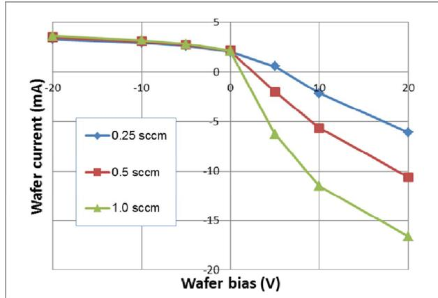
**FIGURE 5.** Net current to a biased wafer with unscanned ion beam, B 5 kV 2 mA, on the wafer. At a few Volts bias the net current to the wafer is zero. PEF power 30 W.
