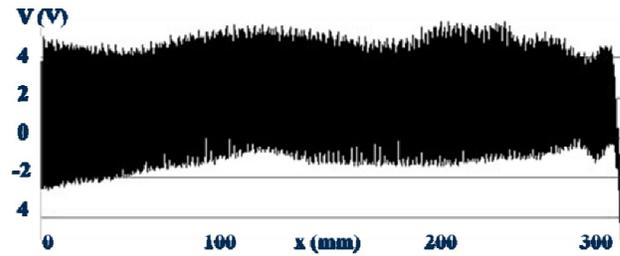
**FIGURE 6.** Charge monitor profile for a 10 keV, 2 mA Argon beam scanned at 100 Hz. PEF flow 0.3 sccm, power 50 W.
