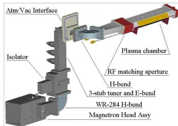
**FIGURE 2.** Components of the microwave plasma system
