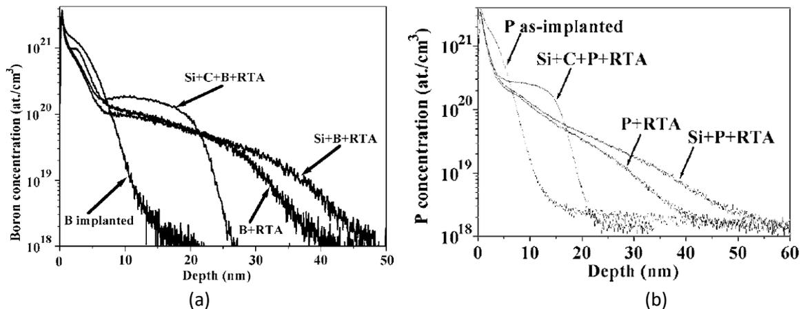
Figure 1: Suppression of (a) 0.5 keV B and (b) 1 keV P diffusion with a C co-implant (6 keV,  $1 \times 10^{15} \text{cm}^{-2}$ ). The B and P doses were  $7 \times 10^{14} \text{cm}^{-2}$ ; the RTA was a  $1050^\circ\text{C}$  spike anneal [71,72].
