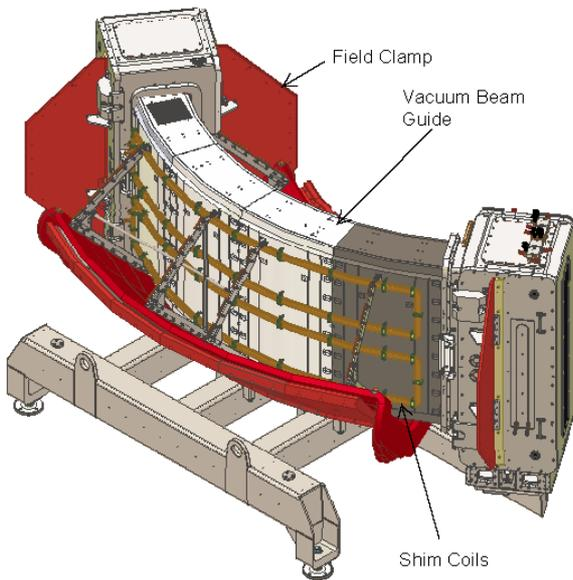
Fig. 24. iG6 with upper yoke segments and coils removed
