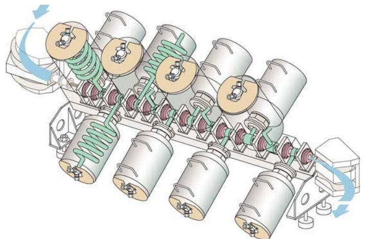
Fig. 7. Sequence of two-gap resonators used in the NV2000.
