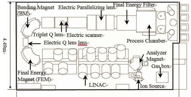
Fig. 10. SMIT ultra high energy S-UHE implanter.
