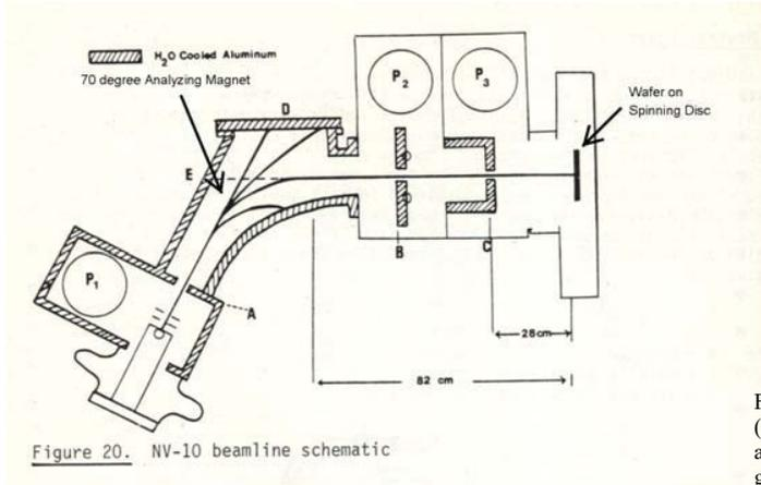
Figure 20. NV-10 beamline schematic
