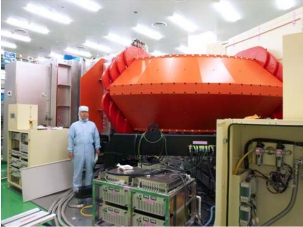
Fig. 23. Nissin iG5 FPD implanter for 1300 x 1500 mm substrate size
