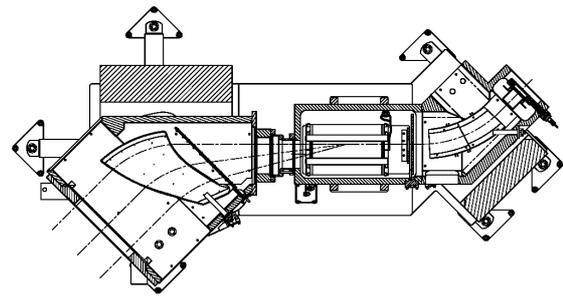
Fig. 14. EX2000 beam line after the post accel/decel lens.
