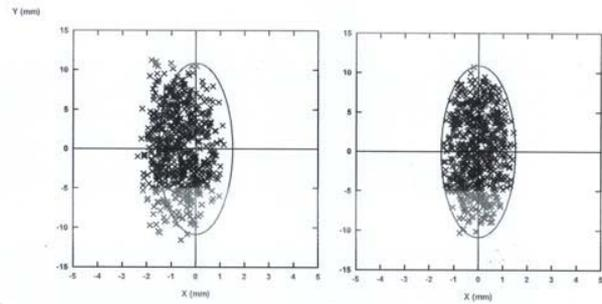
Fig. 4. The NV10 Beam emittance at the resolving slit with (right) and without (left) second order aberration corrections. The pole edge concave curvature at the entrance and exit, in conjunction with the second order term in the gap field, eliminates curvature in the image at the resolving slit and enables a mass resolution of 60-70 to be realized.
