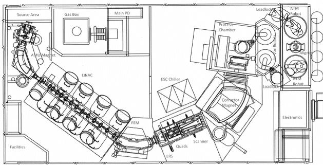
Fig. 9. Purion XE high energy implanter.
