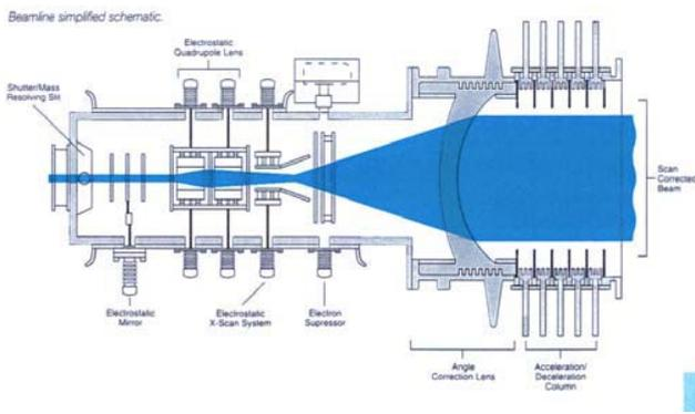
Fig. 16. Electrostatic scanning method used in the NV8200
