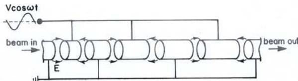
Fig. 5. Sloan Lawrence drift tube linac.
