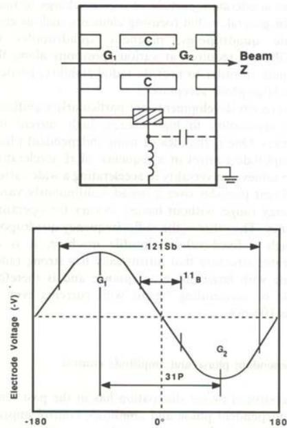
Fig. 6. The two-gap resonator - illustrating its broad velocity acceptance and ability to accelerate particles over a wide mass range.
