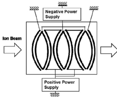
Fig. 11. The electrostatic parallelizing lens used in the SMIT S\_UHE high energy implanter
