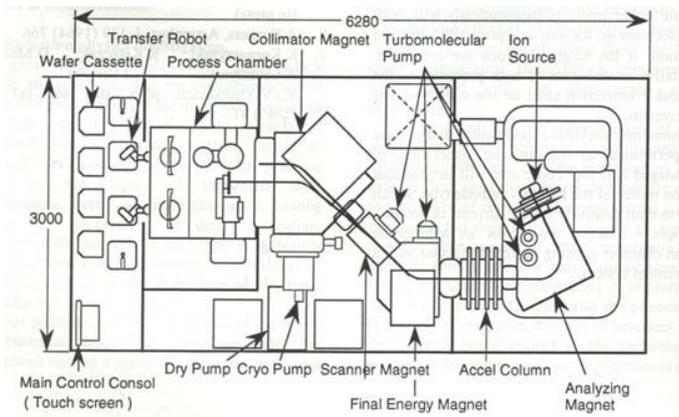
Fig. 13. Nissin Exceed 2000 magnetic scanning beam line.
