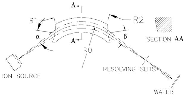
Fig. 3. Schematic of the NV10-80 analyzer magnet pole
