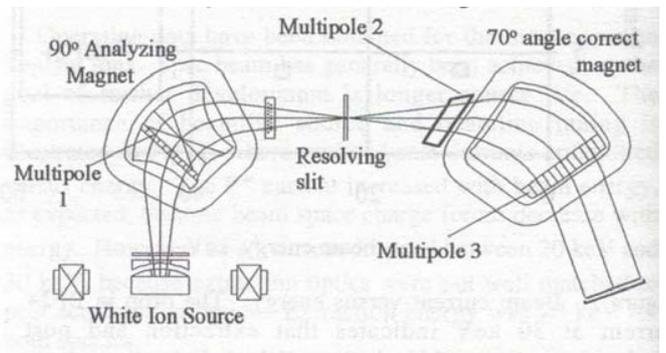
Fig. 18. Beamline schematic of the Varian SHC-80 high current flood ion implanter
