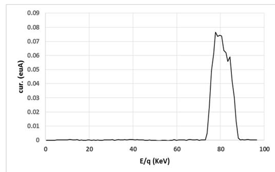
Fig.4. electrostatic rigidity spectrum of high current As++++ beam.
