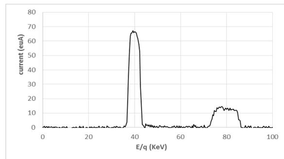
Fig.3 Electrostatic rigidity spectrum of P++++ beam.
