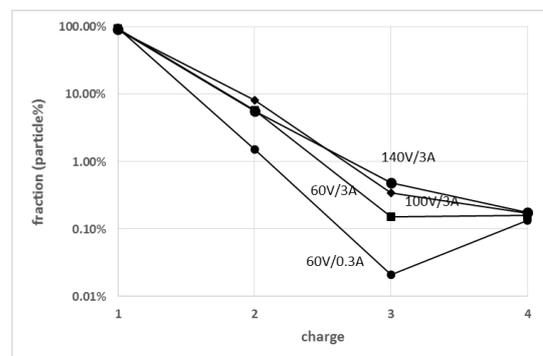
Fig.1. measured phosphorus charge state distributions at four arc conditions.
