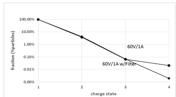
Fig.8 Arsenic charge fractions. With and without the filter.
