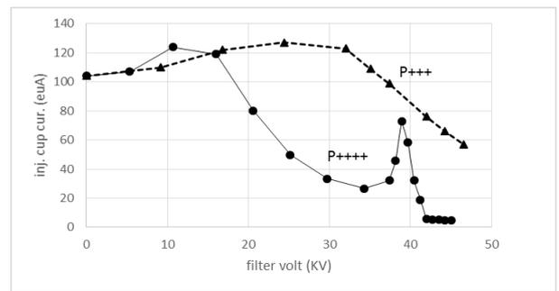
Fig.6. transmitted ions through retardation filter.
