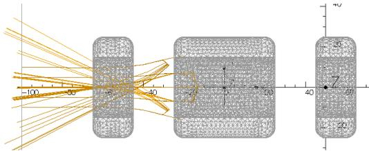
Fig.5.  $E/q=40\text{KeV}$  beam into retarding filter at  $42\text{KV}$ .
