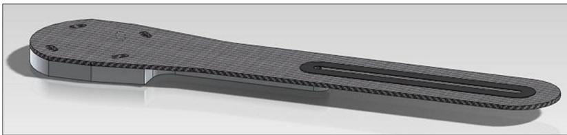
New End-effector Design with Material Designed for Low Metal Contamination
