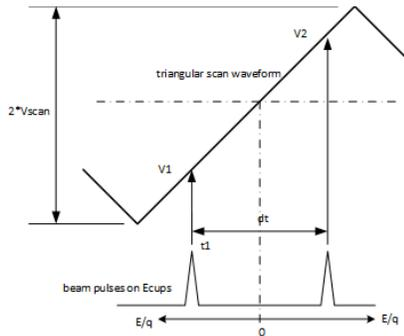
Fig. 4. Pulse timing spectrum from ETS
