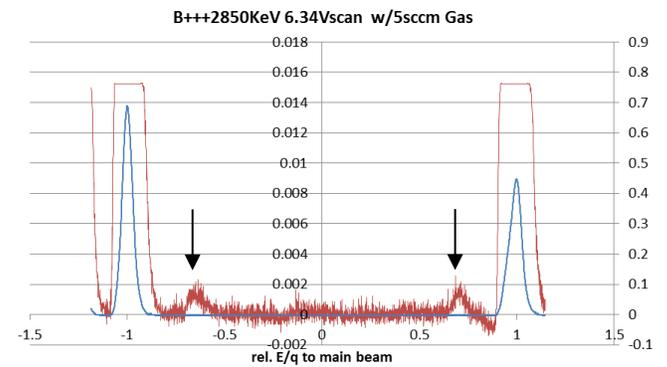
Fig. 6. Time Spectrum from Beam Purity Analyzer on the Forced EC creation.
