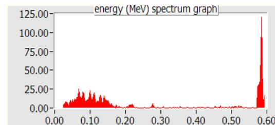
Fig. 1. Typical Output Energy Spectrum from RF Linac
