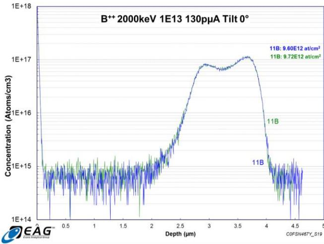
Fig. 7. SIMS depth profile, B++2000KeV, channeling condition
