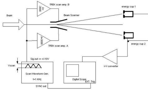
Fig. 3. ETS block diagram.
