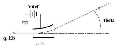
Fig. 2. Basic electrostatic deflector
