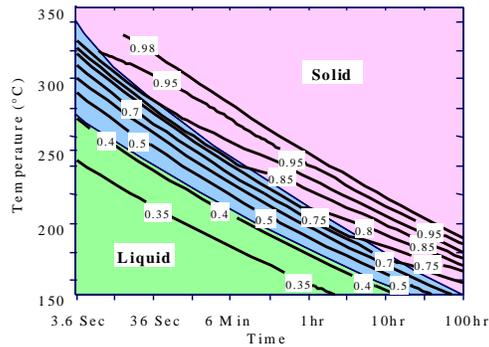
**Fig. 4: TTT diagram for Cyclotene™ polymers.**
