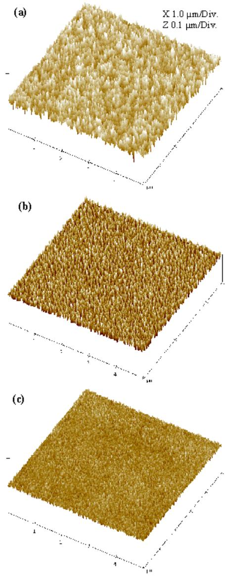
**Fig. 11: AFM images of BCB surface after descum. (a): forming gas only; (b): forming gas with 4sccm  $CF_4$ ; and (c)  $O_2/CF_4$ .**
