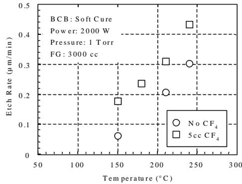
**Fig. 8:** BCB etch rate as a function of temperature with or without CF<sub>4</sub>, obtained on 100 mm patterned wafers.
