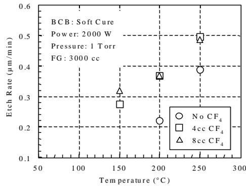
**Fig. 9:** BCB etch rate as a function of temperature with or without CF<sub>4</sub>, obtained on 150 mm wafers.
