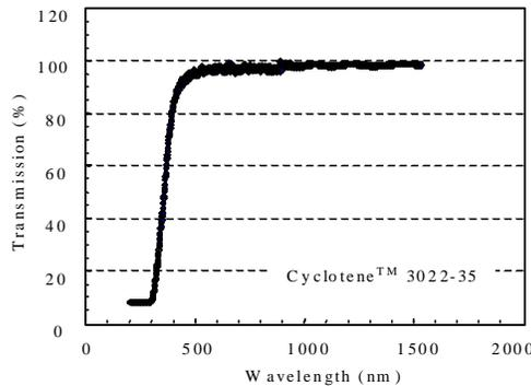
**Fig. 2: Transmission spectra for Cyclotene™ polymer [8]**
