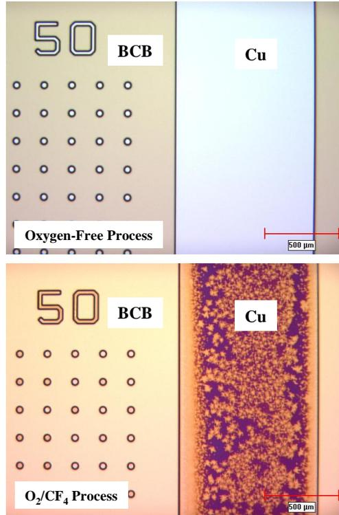
**Fig. 10: Optical microscopy of Cu surface after descum showing severe corrosion of Cu after O<sub>2</sub>/CF<sub>4</sub> plasma descum in contrast to a corrosion-free surface after O<sub>2</sub>-free plasma descum.**
