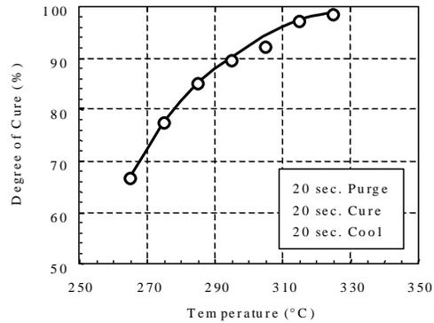
**Fig. 5: The degree of cure versus hot-plate temperature for snap curing process for Cyclotene™ polymer.**
