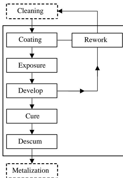
Fig. 7: The process flow diagram which is commonly employed for photosensitive BCB
