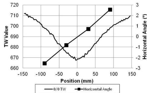
**FIGURE 4.** The horizontal TW variation across a wafer implanted with B+ 60 keV  $2 \times 10^{13} \text{ cm}^{-2}$  run at  $0^\circ$  tilt with the P-lens off. Angles vary linearly from one side to the other.
