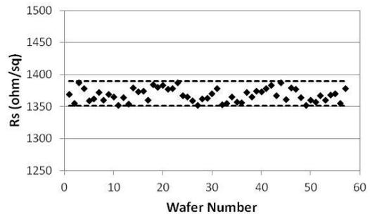
**FIGURE 8.** Sheet resistance results of regular B+ 150 keV  $2 \times 10^{13} \text{ cm}^{-2}$  implants run at tilt/twist of 1°/21°. Upper and lower lines indicate a change in Rs equivalent to +/- 0.3°.
