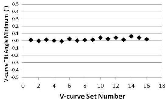
**FIGURE 10.** The wafer implant tilt angle as calculated by V-curve minima of  $P^{++}$  500 keV  $2 \times 10^{13} \text{ cm}^{-2}$  implants. The average angle is  $0.023^\circ$  and the standard deviation is  $0.019^\circ$  ( $1\sigma$ ).
