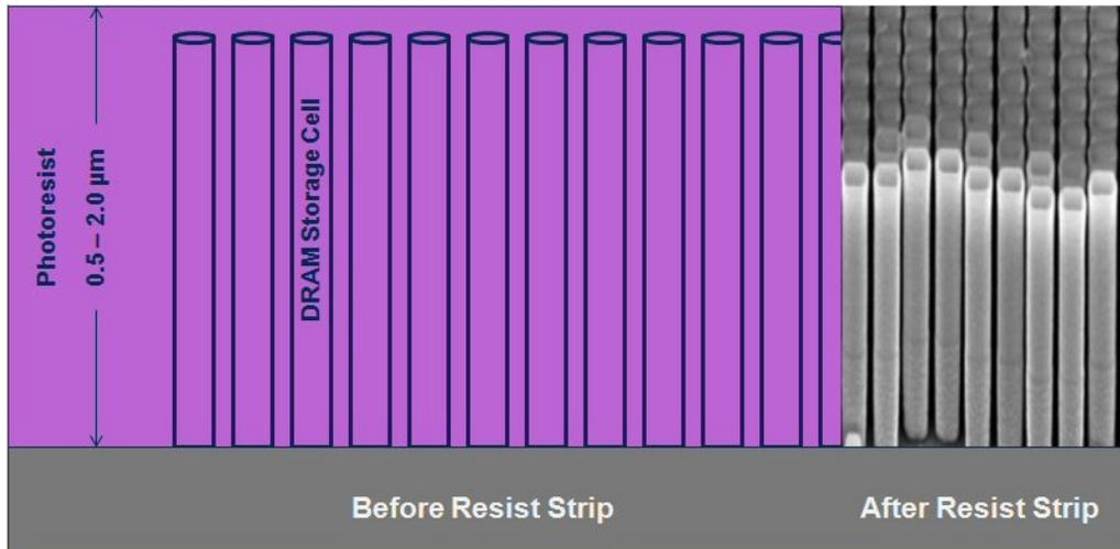
Figure 15. Example of resist removal over an array of DRAM storage cells. The DRAM capacitor cells have aspect ratios of > 20:1 causing significant thickness being deposited inside the cells during the masking process. Removal of this resist requires extremely high selectivity to avoid etching or oxidation of the storage cell electrode material, in this case TiN.
