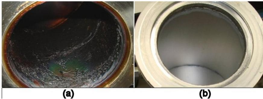
Figure 4. Example of cracked photoresist deposits in the vacuum line of a system running 1000 photoresist coated wafers using a forming gas (FG) plasma strip process (a) versus a system running an  $O_2+FG$  process (b). The FG process is a mixture of 4%  $H_2$  in  $N_2$ .
