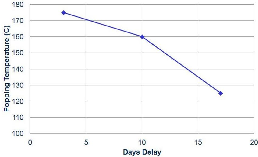
Figure 12. The measured popping temperature of a DUV photoresist as a function of the time delay after ion implantation. After about 2 weeks delay, the popping temperature is significantly reduced. For some resists, popping can be observed at room temperature after several weeks of sitting in cleanroom air.
